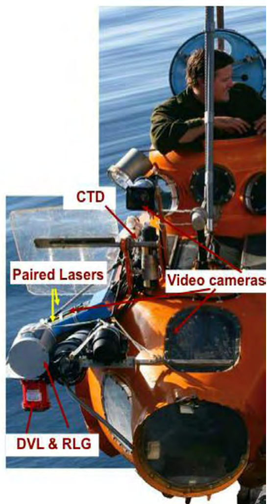
Figure 21. The yellow Delta (right) and red Dual Deepworker (left) research submersibles accommodate one scientific observer and one pilot, and were operated to a maximum depth of 365 m (Delta) and 440 m (Dual Deepworker) at a survey speed of 0.5-1.0 kts.
