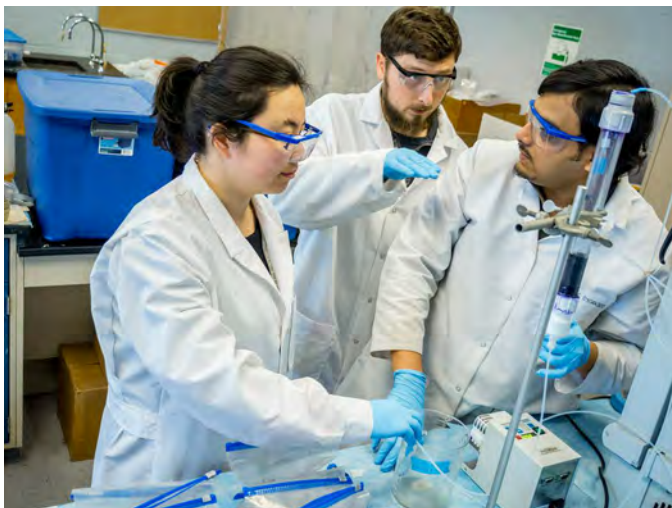
Laboratory column studies using aluminum-based drinking water treatment residuals. Photo - Mike Peters, MSU
