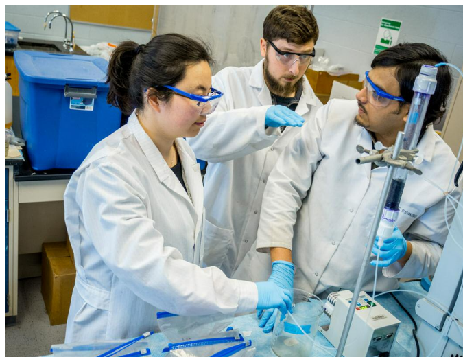
Laboratory column studies using aluminum-based drinking water treatment residuals. Photo - Mike Peters, MSU
