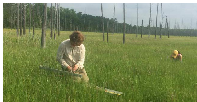
Measurement of coastal marsh elevation change using a surface elevation table, or SET. Project scientists are monitoring marsh elevation change and sediment deposition at more than three dozen locations in regional estuaries. This photo also shows how marshes are migrating into coastal forests with sea level rise, resulting in a 'ghost forest' with a marsh understory.
