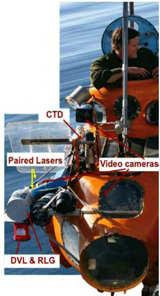
Figure 21. The yellow Delta (right) and red Dual Deepworker (left) research submersibles accommodate one scientific observer and one pilot, and were operated to a maximum depth of 365 m (Delta) and 440 m (Dual Deepworker) at a survey speed of 0.5-1.0 kts.
