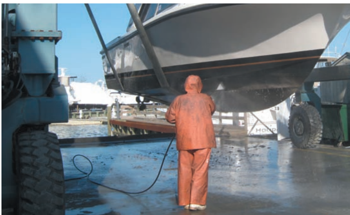
Wastewater from the pressure washing of boat bottoms can contain materials that are hazardous to the environment and should be managed properly with a storage or treatment system.
