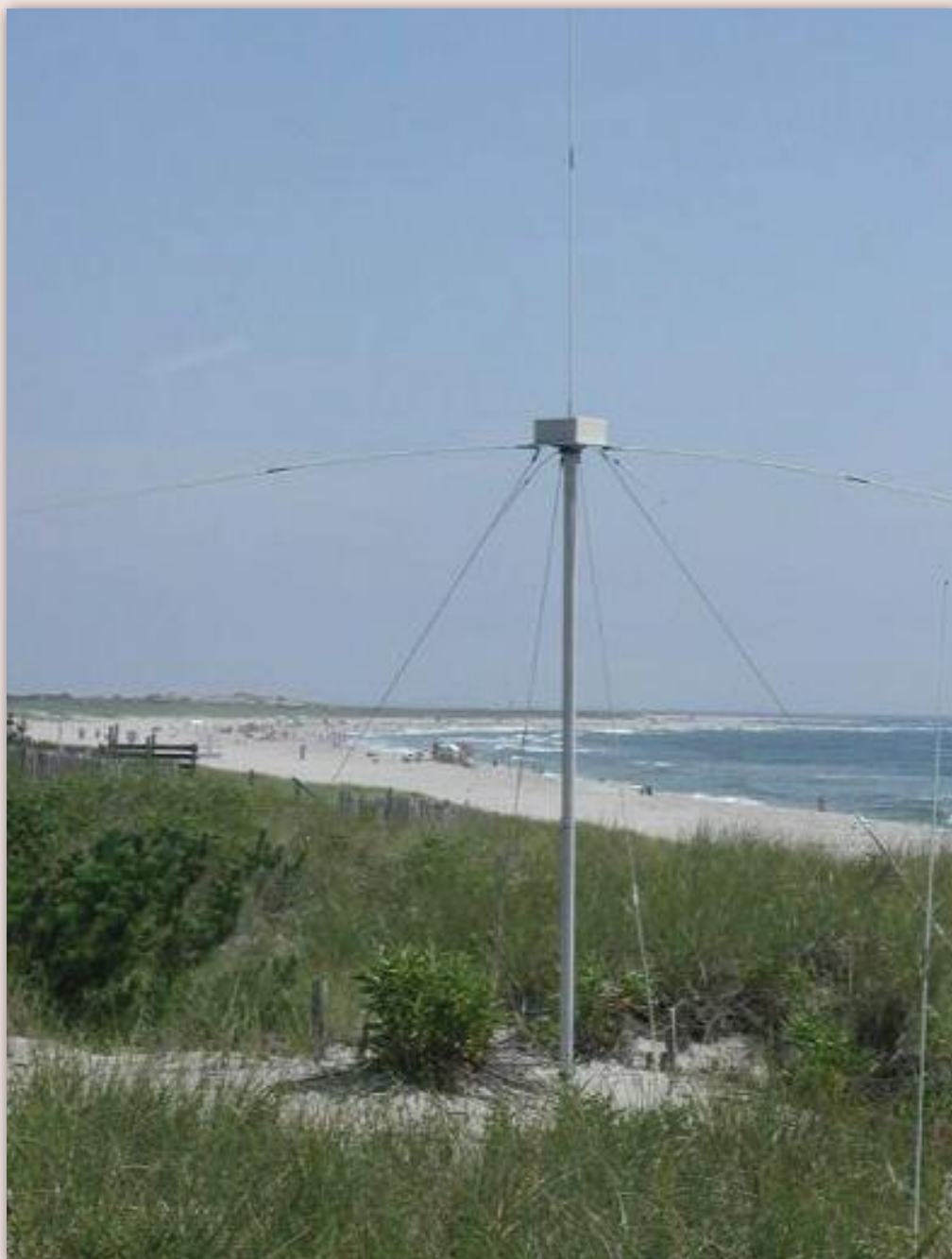
High frequency (HF) radars remotely measure waves and currents, allowing researchers to monitor conditions along the coast.
