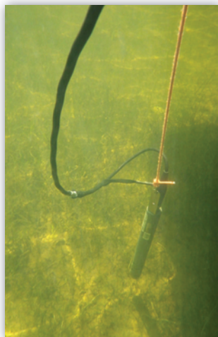
YSI probe measuring temperature, salinity, dissolved oxygen and pH in the seagrass bed
